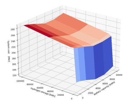
Figure 29: System cost analysis of storage combinations in Ekeröd with one hectare solar panels
