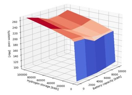
Figure 30: System cost analysis of storage combinations in Ekeröd with five hectare solar panels
