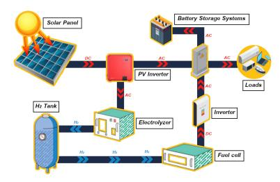
Figure 6: Hydrogen storage system together with battery, generation and load [18]
