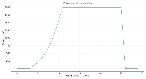
Figure 15: Power curve for the chosen wind turbine
