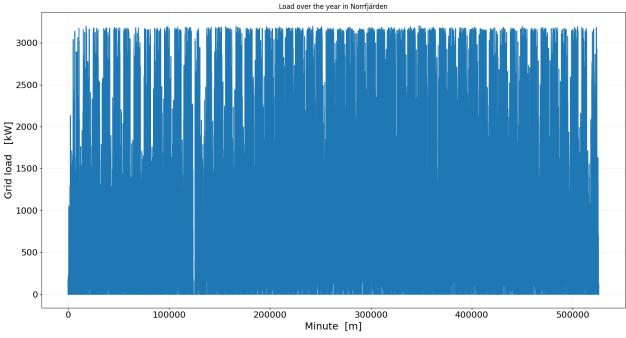
Figure 46: Grid load in Norrfjärden with no local generation or storage
