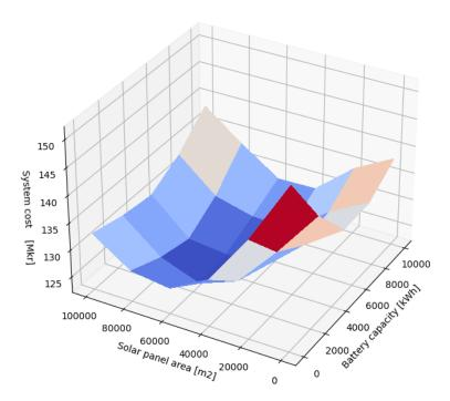
Figure 33: System cost analysis of battery and solar panel combinations in Ödeshög
