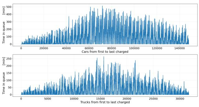
Figure 27: Queue times in Norrfjärden with 20 car and 3 truck charging spots but 60 km between charging stations
