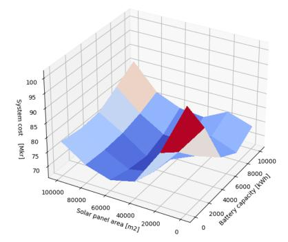
Figure 32: System cost analysis of battery and solar panel combinations in Ekeröd
