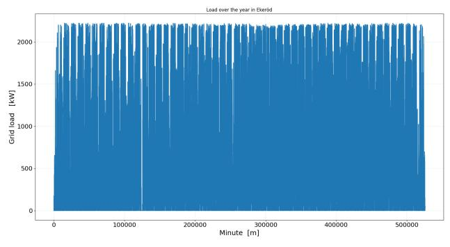
Figure 44: Grid load in Ekeröd with no local generation or storage
