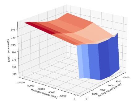
Figure 28: System cost analysis of storage combinations in Ekeröd with 0.5 hectare solar panels
