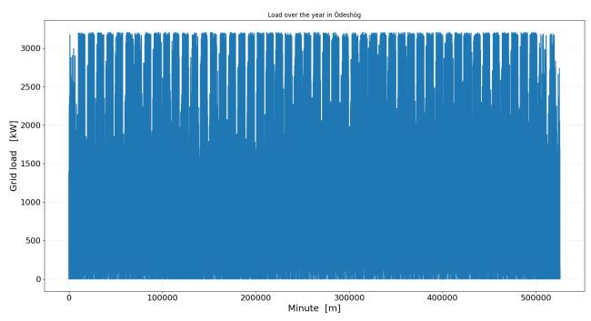
Figure 45: Grid load in Ödeshög with no local generation or storage
