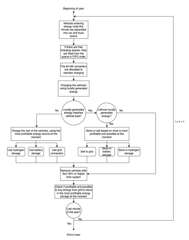
Figure 21: Flow chart over the simulation process
