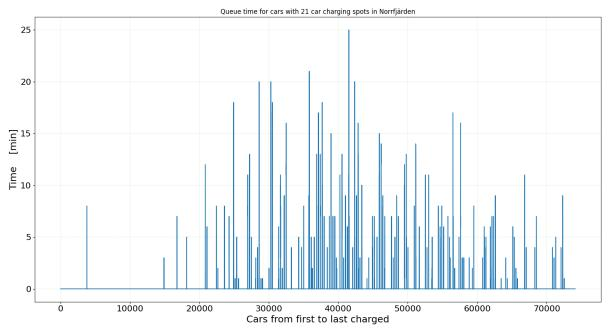
Figure 23: Car queue times in Norrfjärden with 21 car and 3 truck charging spots
