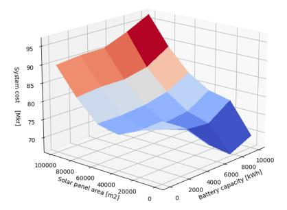
Figure 34: System cost analysis of battery and solar panel combinations in Norrfjärden
